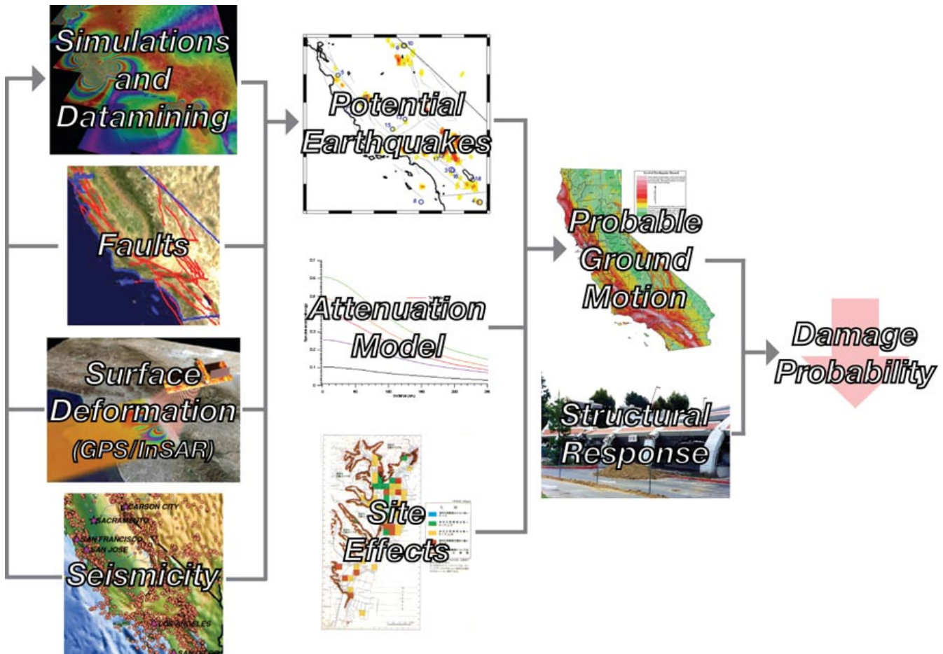
Figure 1 – Risk estimation processing showing the relation between a geophysical sensor web and earthquake risk mitigation. The sensor web is on the left column and feeds into simulation and data mining tools. These in turn flow down and combine with other inputs to produce an estimate of damage probability.
